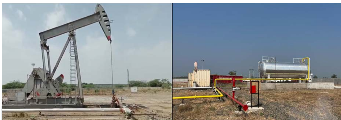
Surface Production Unit (Sucker Rod Pump and Crude oil Storage tank) at Galiyana#1 Quick Production System (QPS) in the block CB-ONN-2010/11. Commencement of Commercial Hydrocarbon Production by 3rd Indian CPSU as operator.
