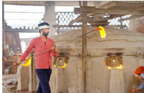
Skilful handling: A worker carries red-hot gobs of glass on a long, metallic pipe at a glass factory in U.P.'s Firozabad. RICHARD KUJUR
